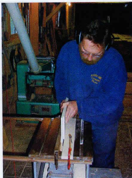
Cutting the frame rest rabbet with a dado blade.
