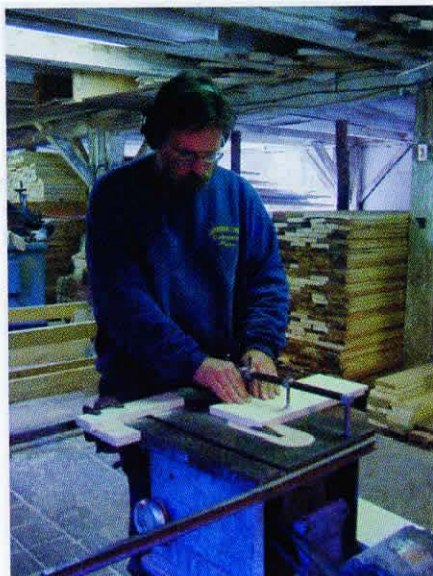
The rabbets are cut with the miter gauge. The board clamped to the saw table automatically positions the stock for milling.
