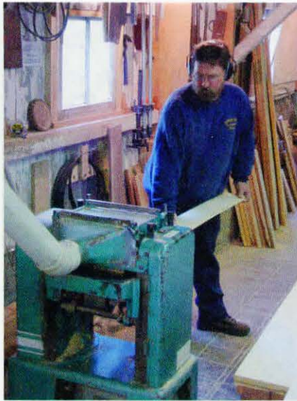
With one face flat, the lumber is planed to 3/4"
