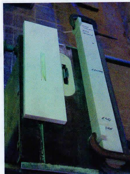
Handhold cut with the dado blade showing the fence setup.
