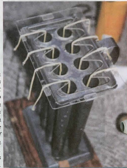
Then, Nancy's secret. A thin piece of plexiglass was cut to fit the inside of the molds' top. When in place, the 'points' with notches will be exactly centered over the cavity to be filled with wax.
