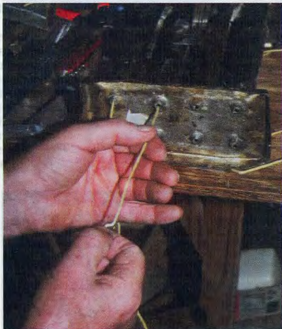
An evenly waxed wick, with no spots without wax, threads easily. Miss a spot and the wick will bend and twist and be nearly impossible to thread.
