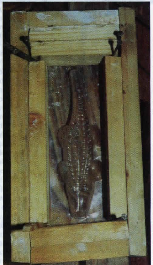
This is the box made to make a Gator mold. It comes apart easily, and the final product is shown on the opposite page.
