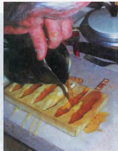
When pouring small molds a tin can, with a pinched nose makes an inexpensive container. Keep it warm, but not so warm you burn your fingers.
