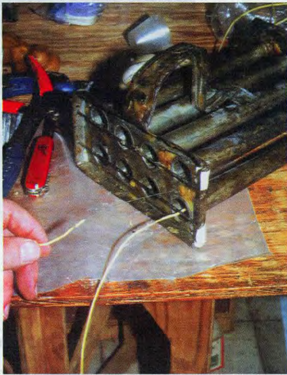
Frame wire, when wrapped around the waxed wick and twisted so it is in line with the wick will make threading the wick from the large end of the mold through the small end much, much easier.
