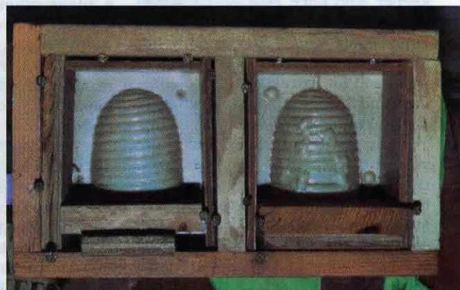
A home made candle mold maker. Oil well before placing the plaster in to set.
