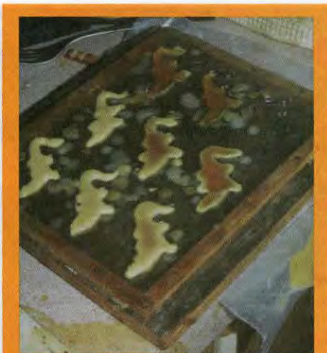
Thin plastic candy molds can be used, but won't last long. To make them stable when hot wax is in them, provide a foundation underneath for support and a frame around the top to keep the mold from curling.
