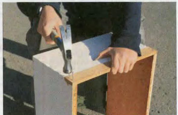
Nail it in but pre-drill the holes first.
