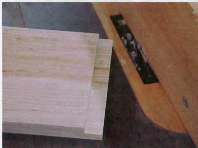
A dado cutter head and one rabbet cut.
