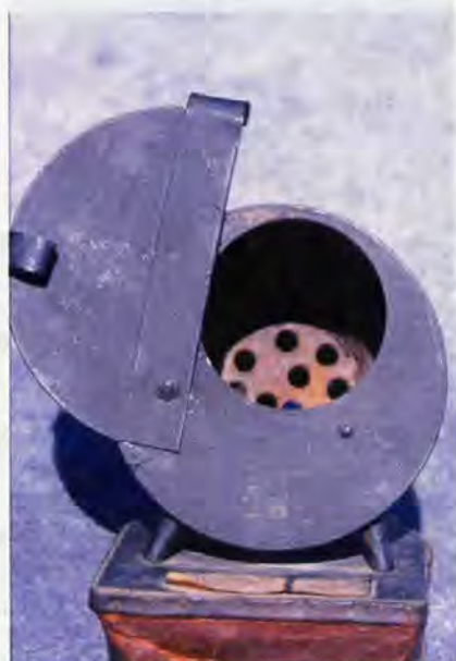
Figure 3: The older style holes in the fire grate. these are the larger holes that let the sparks fall on the bees. To get an idea how big these holes are, compare them with the holes in the fire grate of your modern smoker.
