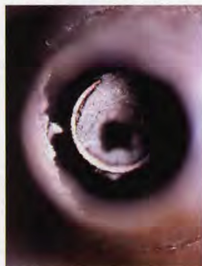
Figure 2: Looking into the funnel of a Clark smoker. The blast tube (in the middle of the picture) is almost completely filled with a light gray deposit. This is the large size blast tube. Small size tubes show the blockage even more acutely, but they are recessed further back in those smokers and were too difficult for me to photograph.
