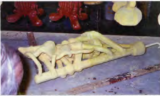
#3. The ceramic shell around the wax statue; note the pouring cup, sprues, and vents.
