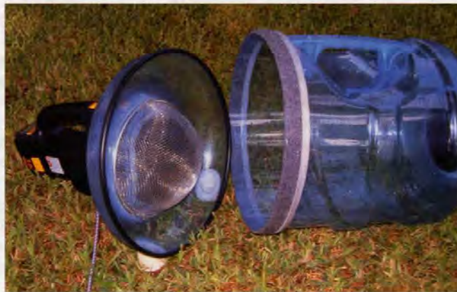
The disassembled unit, (from left to right) the vacuum and inside screen attached to the removable bottom, with the black plastic automobile door protector; the larger section, showing the felt weather stripping and white foam seal.
