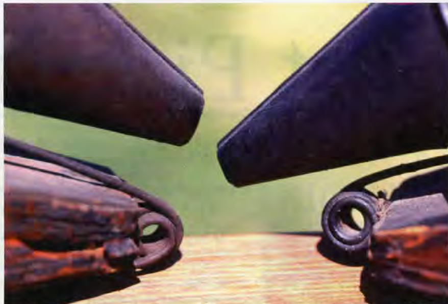
Figure 4: Comparing two versions of Clark smokers. Note where the funnel ends in relation to the spring coils. The older one has the funnel protruding past the spring. The newer one has the funnel even with the spring.
