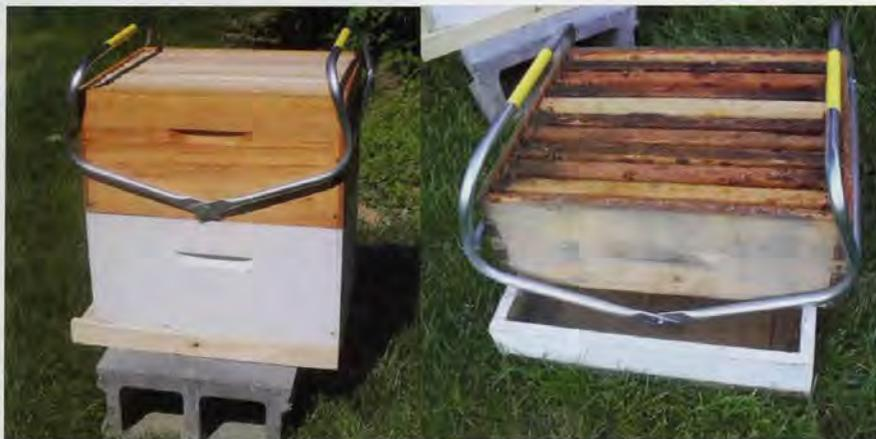
This tool may be used on all sizes of hive bodies. The brood box has plenty of depth so the tool does not stick below the box. That makes it easy to set down most anywhere. With the medium and shallow boxes just set the first box crossways on an inverted hive cover or another box to make sure the bottom of the hive tool is clear. This tool was designed to make it easier to lift single boxes with weights up to 70 pounds or more. This tool was not designed to be used over an outer cover.
