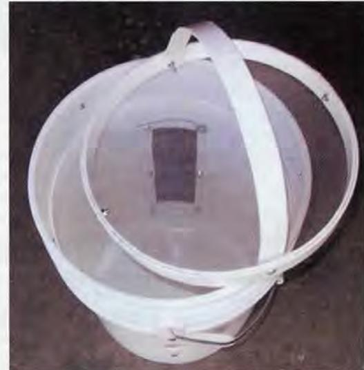
Screen Divider - Ring #four on the inside, ring #one on the outside. Screen in between four and one. Ring #three as handle.
