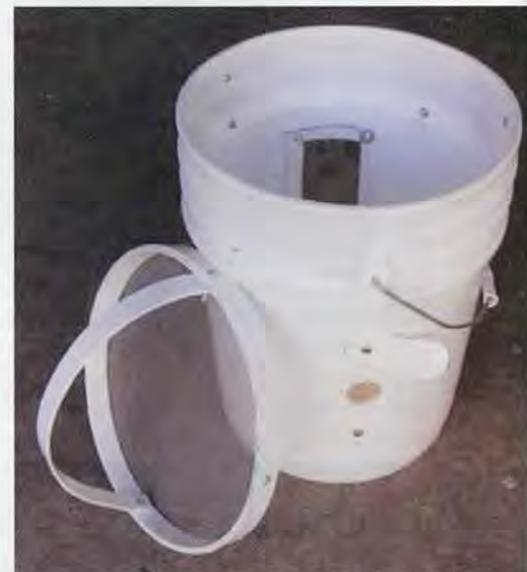
Screen cover on outside. Ring #two positioned inside pail. Hole for vacuum hose with hole cover in place.
