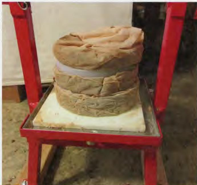
*Winepress can be used as either a cloth and rack press or as a basket press with spacer plates to make it more efficient like a rack press. Wine press with apple scatterer converted to a rack and press setup or with spacers used in press basket to make it much more effective than just pressing a single big bag (basket removed to see configuration of spacers and bag).*
