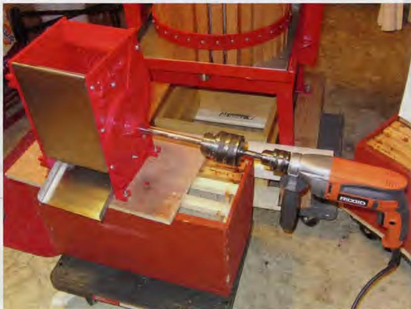
*Scatter, which chops the whole apples into little bits, run with a drill that has a lockable trigger is much faster than the handwheel. Next upgrade an electric motor and pulleys.*
