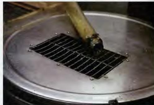
*Honey drains from our 50-frame extractor into the sump and is pumped into settling tanks.*
