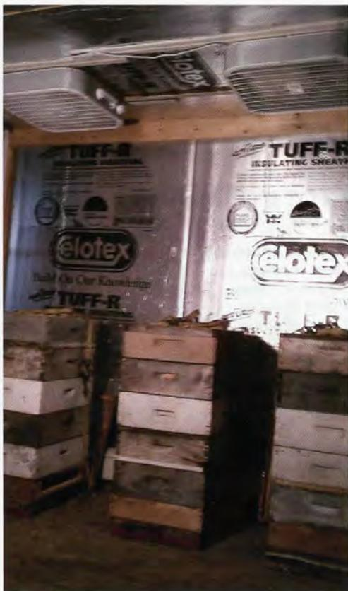
Several large fans, in Richard Linck's hot room, force warm air down through honey supers and out through screens in the ventilation boxes, on which they are stacked, to remove moisture which, in turn is
