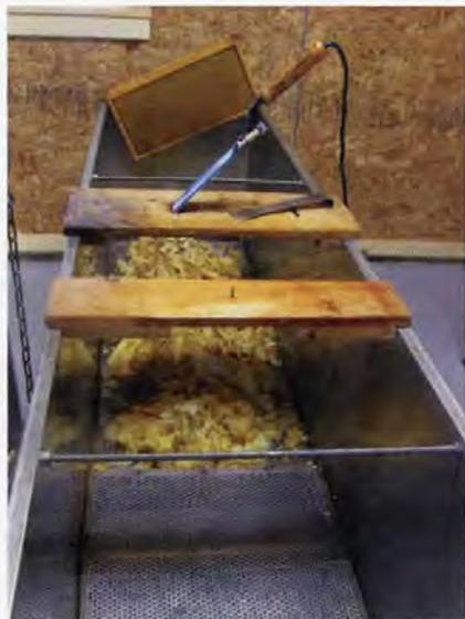
*This extra large uncapping, holding tank will contain several days cappings which drain through a screen, reducing the amount of honey going into the wax melter.*
