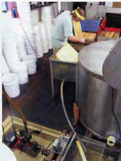
*Our set-up in Interlaken, NY is simple. Here Christopher Waid scratches open some cappings that were missed by our uncapper before placing the comb in holding tank to await extraction.*
