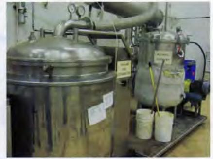
where the alcohol is removed, leaving only the very hot propolis which is still a liquid.
