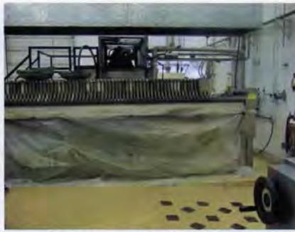
into a pressure filter to remove even the tiniest of foreign objects. When filtered, it is again pumped to a distilling tank
