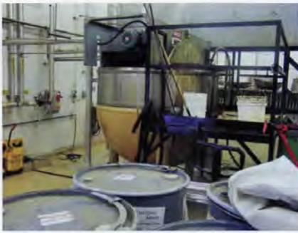
This material, usually mixed with some amount of wax and other foreign material, is placed in a large tank. Alcohol is added and the propolis is dissolved. The liquid propolis mix is pumped out of the tank
