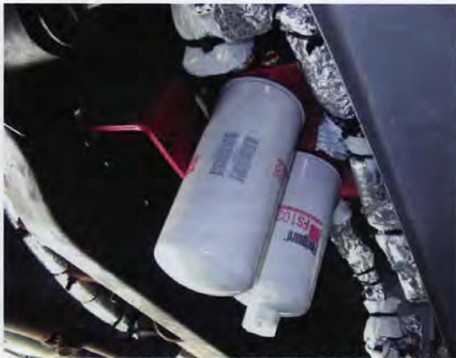
The Fass Fuel filtering system includes a fuel pump that pumps the veggie oil from the fuel tanks, through the filter and up toward the engine.
