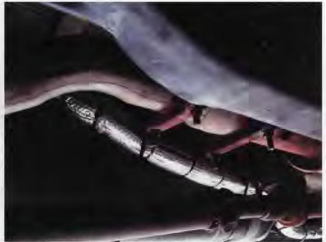
*Due to the cold temperatures in Winter, the vegetable oil fuel lines and the antifreeze lines that run between the engine and the fuel tank in the truck bed have been bundled together and wrapped with insulation.*
