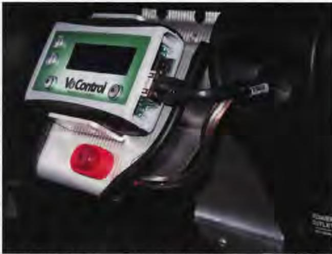
*The brains of the vegetable oil fuel system, the VO Controller is mounted on the dash where the ash tray used to be. The hole for the cigarette lighter was used to run the wiring to the controller. The large red button is hooked up to a heating pad that is attached to the bottom of the fuel tank in the truck bed in order to provide additional heat in Winter.*
