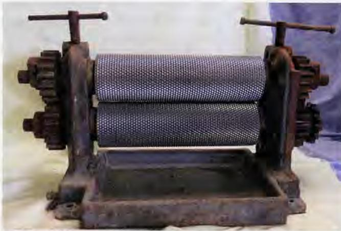
*Small set of commercial foundation rolls for regular worker cell foundation.*
