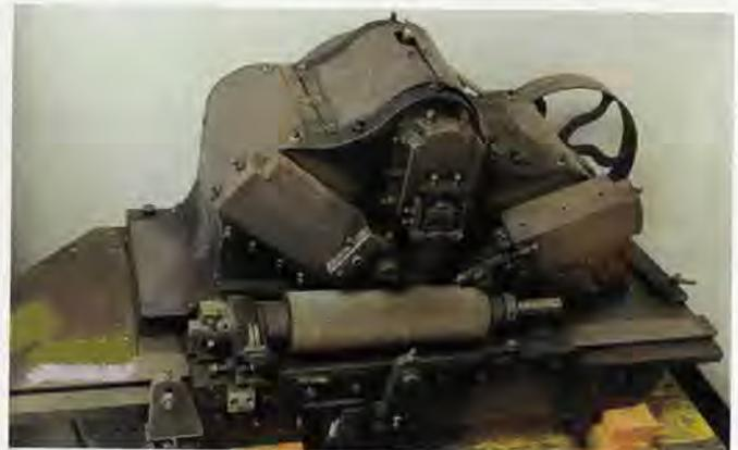
**Milling Machine that makes foundation rolls.**
