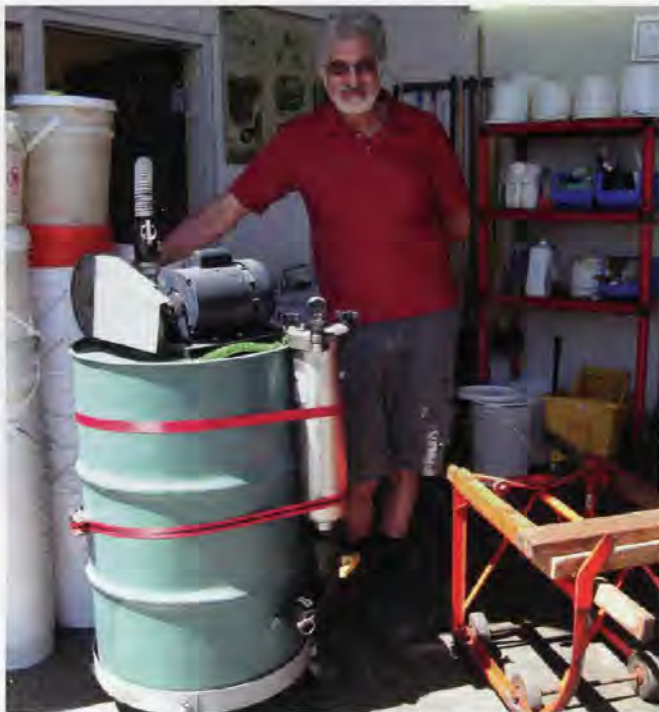
Ishai Zeldner with the pump that moves honey from the warming room into the bottling room, through a light filter at the Z facility.
