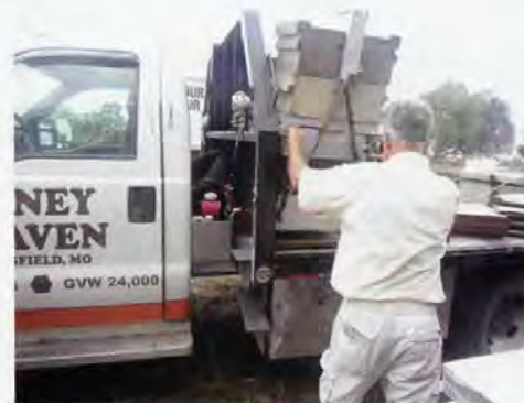
Once off the trailer, the stack is swung over to the truck and gently set down, exactly where it should be.
