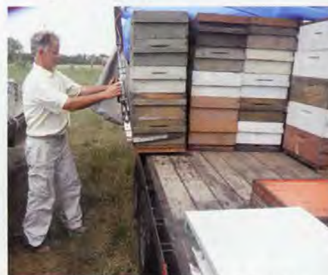
. . . and slid in. Each super has a cleat that the fingers of the cradle fit under. When the cradle is snug against the front of the stack the up button is pushed and the stack is lifted.
