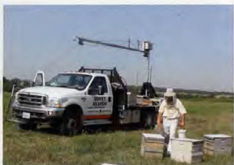
The boom is mounted on the back of the truck. The long arm turns 360 degrees, and the pulley lift on arm slides the entire length of the arm. Moving the cradle up and down is mechanically driven, moving the slide is done by the beekeeper.
