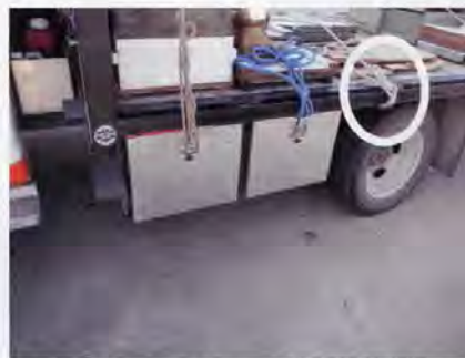
A good bee truck comes equipped with a bar on the side of the bed for tie-downs, and lots of equipment boxes underneath, not taking up important carry room on top. Boxes haul rope, smoker fuel, extra protective equipment, fire extinguishers, tools for engine repair and in this case boom repair, and anything a beekeeper will need when on the road.
