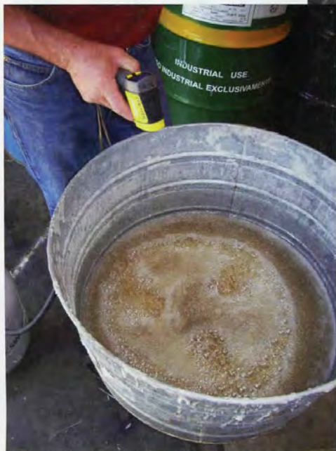
Using a candy thermometer or handheld infrared thermometer, bring the mix to 240 degrees, turn off the heat. Let cool to about 180 degrees.
