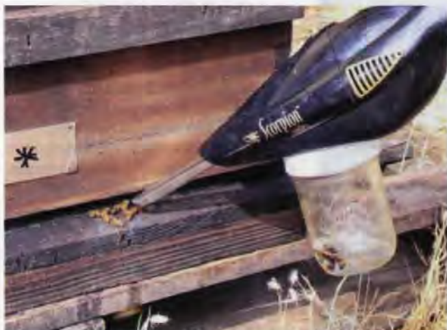
The Suck-a-Bee – a portable vacuum modified to collect bees directly into alcohol. Plans for this timesaving device are at www.scientificbeekeeping.com .
