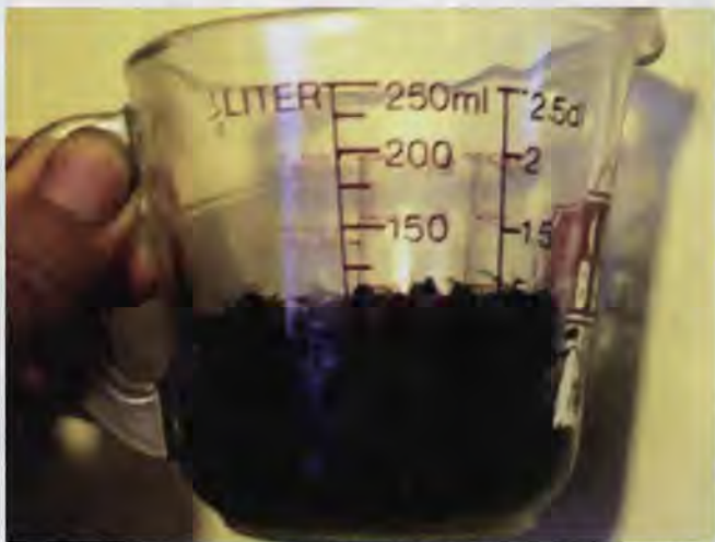
A quick volumetric method of "counting" the number of drained bees in a sample. There are roughly three bees per milliliter. So this sample of 100ml of bees would contain about 300 bees, and need 300 ml of water to dilute them for a standardized spore count. In general, use 3x the volume of water as settled bees.
