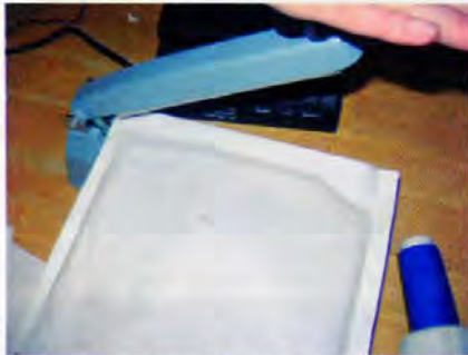
Sealing the 'envelope' with the impulse sealer.
