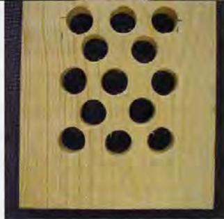
**Step 13:** Cut the frame stabilizers (parts 13) and drill the holes in them. These are used to provide a path for the bees to get to the water on the bottom of the swarm box and to keep the frames from moving.
