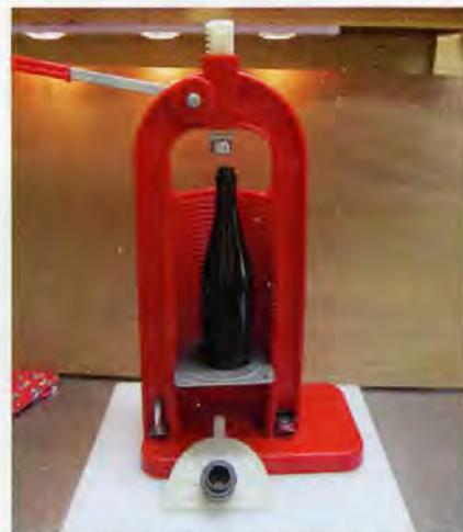
*Colonna table top corker and capper, white part at base is the corker along with the plunger on the left of the base, and a small and large beer capper. Easily adjusts to any bottle size.*
