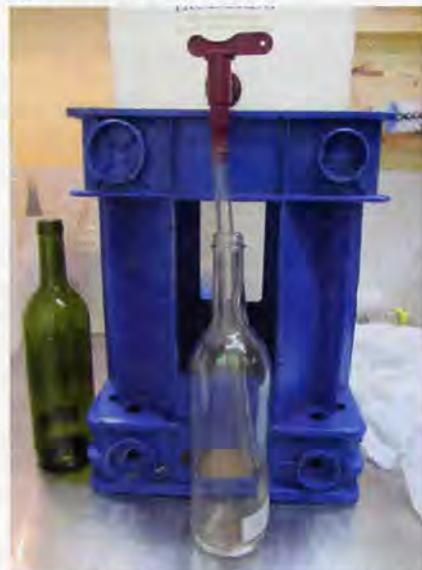
*Bottling bucket with hose attached to spigot. Lift bottle up so hose is on bottom of bottle to decrease oxidation and foaming.*
