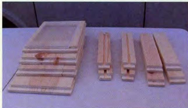
2. To make the window in one side of the bee box, cut 1" strip from the top and bottom of one 11 $\frac{3}{4}$ " piece. From the center strip, cut a 1 $\frac{3}{4}$ " piece from the rebated end and a 1" piece from the opposite end. Now make a 5/16" deep saw cut in the edge of the four pieces to receive the plastic glazing window. Then from the remaining material, cut four 2" x 2" triangular feet.
