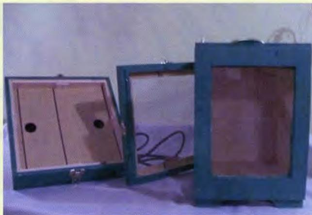
13. Now, final assembly! Attach the vacuum motor to the top of the vacuum chamber. Attach two latches to the vacuum chamber and screen frame and two to the screen frame and bee box. Attach the pivoting covers over the air vents and the hole for the bee hose. Attach the handle on the side with the bee hose.
