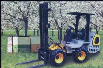
1K Super Bee features planetary drive axles each rated at 8,000 lbs., rugged articulation frame joint, ergonomic operator station and a transverse mounted engine for easy maintenance and service. Call for a spec. sheet or visit [www.nmc-wollard.com](http://www.nmc-wollard.com).
