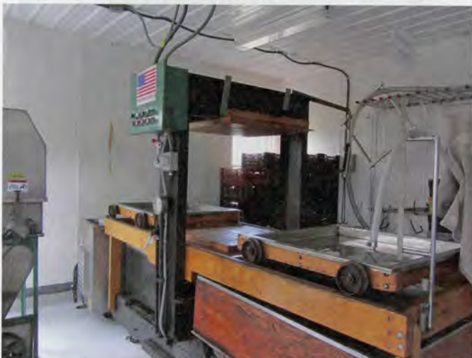
Rob's Rack and Press cider press. Ground apples are layered in cheeses between pressing plates wrapped in special pressing cloths. Some of this cider is being fermented with Charles local raw honey for the first time at DLC.
