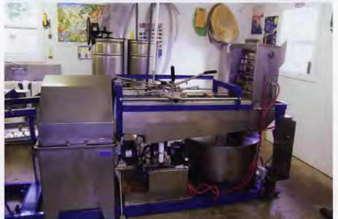
*Carl's compact unit is uncapper on left, wax spinner below, frame holder in the center and parallel radial extractor on the right.*
