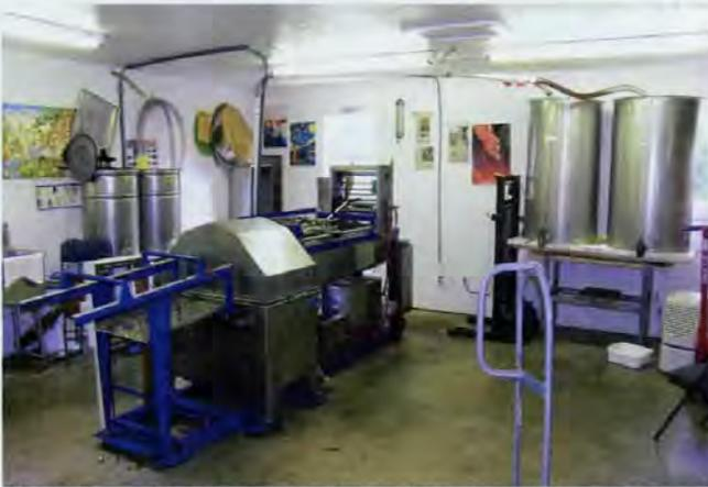
Uncapper, extractor pipes and storage tanks. This arrangement makes it easy to keep honeys separated.
