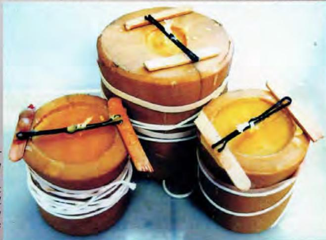
*Poly molds are our choice for making novelty candles. Note that extra wick is wrapped around mold so that they are restraining as candle is removed.*
