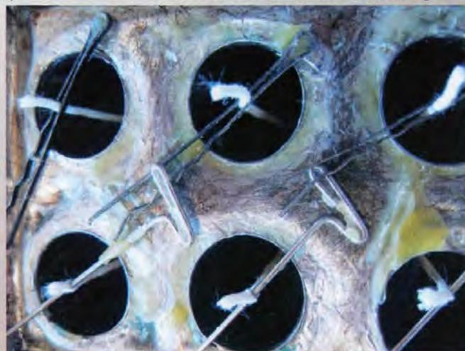
*Metal molds are threaded by pulling wick down thru one tube then up thru the other, being secured by sewing pins and hair pins.*
