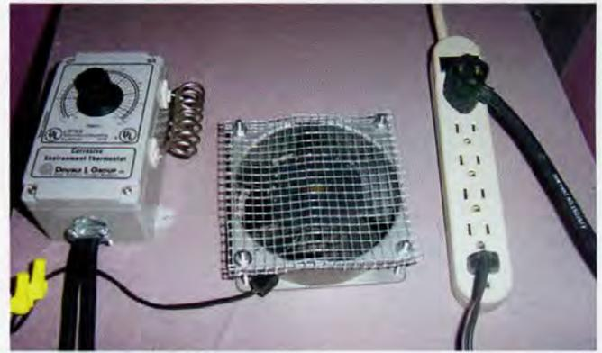
**Hint:** Set the temperature indicator (scale) as per instructions that came with the thermostat before testing the assembly.
