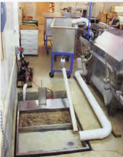
Moveable cappings honey box on stand showing pipe to sump; and extractor, showing large pipe to sump.
