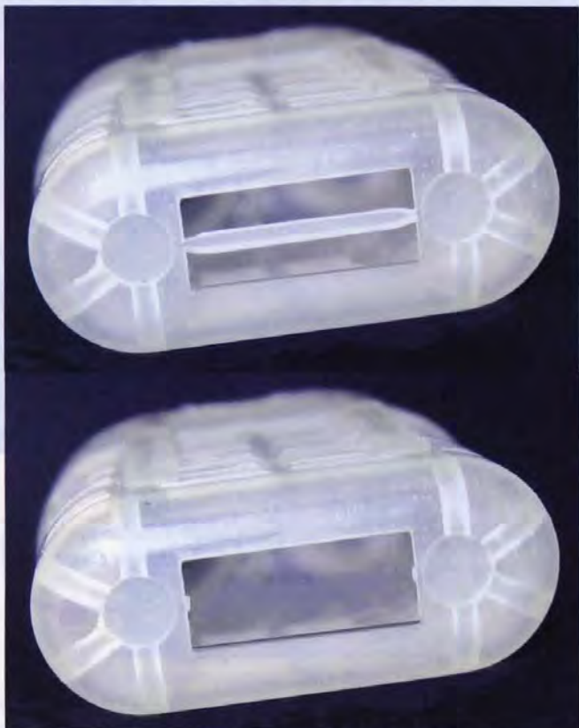
Cage opening with bar place (top) and removed (bottom).
