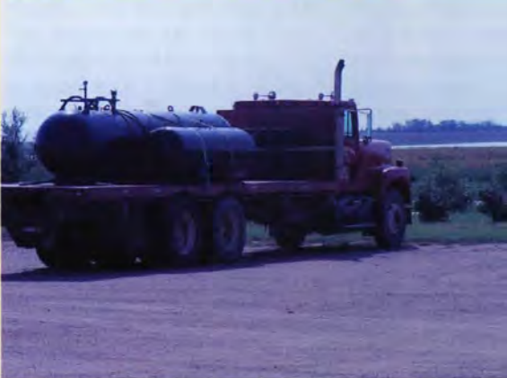
Feeding tank with 500 gallons syrup and 100 gallon air tank.
