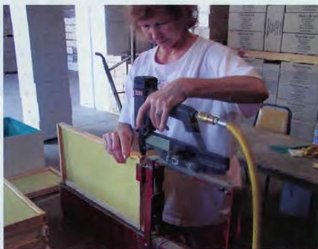
Frames are assembled, glued and stapled . . . by the thousands.
