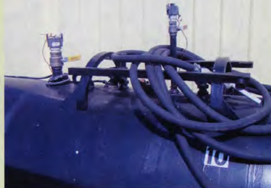
Compressed air is fed into the feeder tank, and it pushes out syrup.
