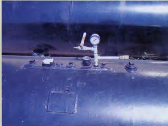
The air-loading system. The field shut-off to the feeder tank is easy to use.
