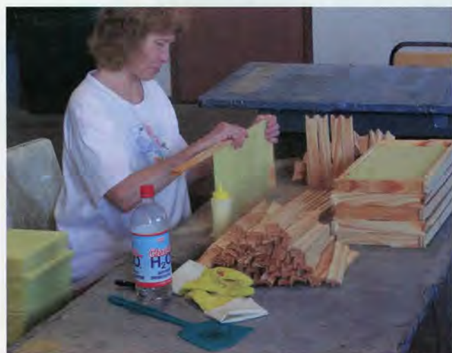
Frames are assembled, glued and stapled . . . by the thousands.
