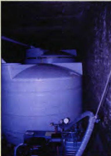
A sophisticated mixing tank is used to mix syrup and water to an exact formula.
