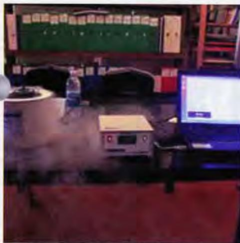
*Cryopreservation in action. Semen samples are in the small black unit in the liquid nitrogen filled "cryobath" on the left. The computer is used to control the freezing rate.*
