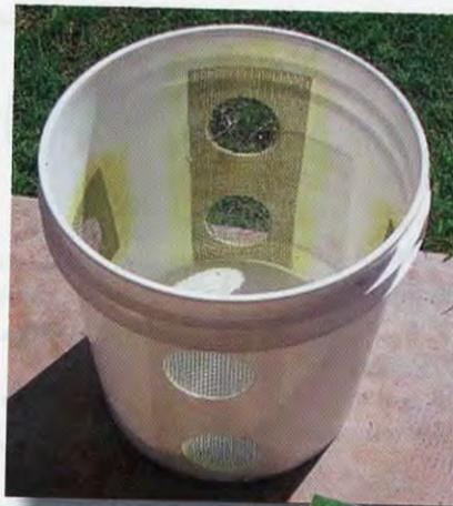
**9.** If you use the vacuum often, you can also attach the screen to the inside of the bucket by using Epoxy glue. The Epoxy comes in all types and applications, so be sure and use one that will work with metal and plastic.
