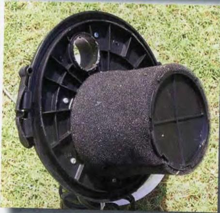
**12.** You will have to cut off the angle piece located on the underside of the vacuum. This allows the bees to fall directly into the vacuum cage and not hit the angle piece.
