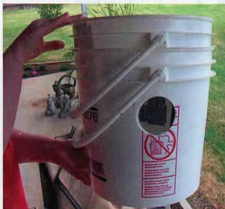
3. Underneath the handle alignment, drill a hole through both buckets using a door knob drill bit . . . 2-1/8 size.
