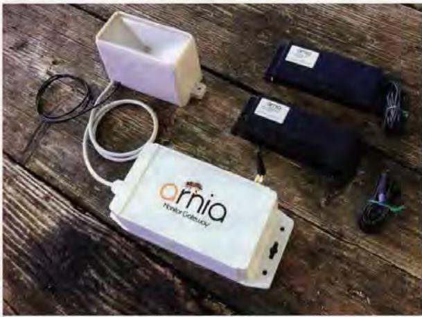
**Figure 3.** arnia Hive Monitors and Gateway unit with weather pack.
