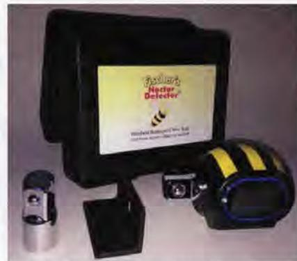
Fischer's Nectar Detector is the result of nearly a decade of effort to find a simple, reliable, low-cost method of weighing every hive a beekeeper owns, quickly, and with minimal effort.
