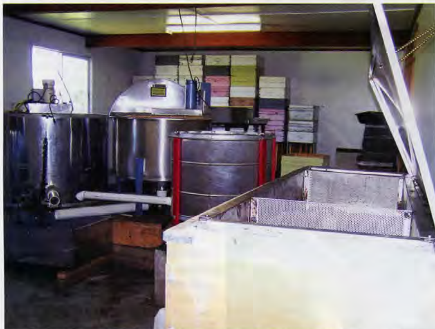
The Honey House. Supers in back came in through the door on the left. Two extractors, left and center, and wax spinner right, with cappings melter in foreground. Sump bottom left. Bottling tank just to the left of sump, out of picture.
