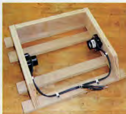
Attach the lamp bases to the sides of the platform.
