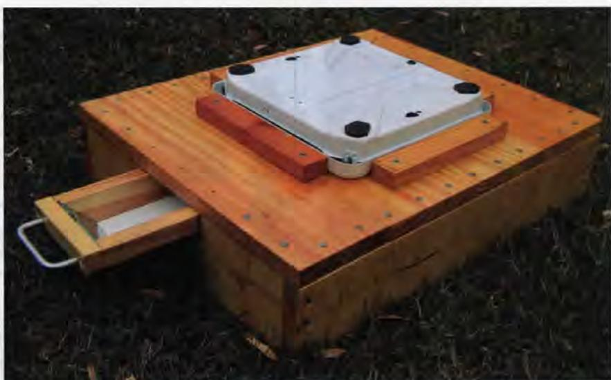
The base with the scale placed upside down and located with four wooden blocks. The periscope is pulled out to the weight reading position.
