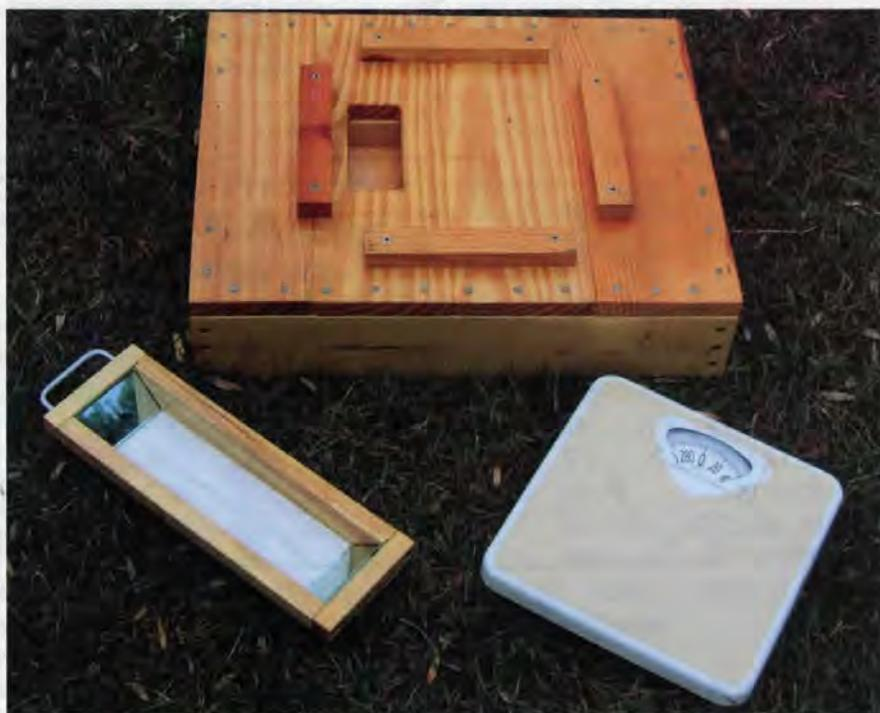
The hive scale base, periscope and standard spring type bathroom scale.
