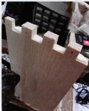
Figure 4: glue on the interior super joint during assembly. (David MacFawn)
