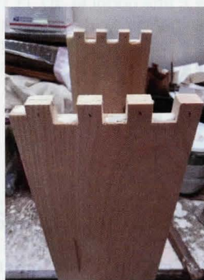
Figure 5: Glue on super joints; note handhold orientation (David MacFawn)
