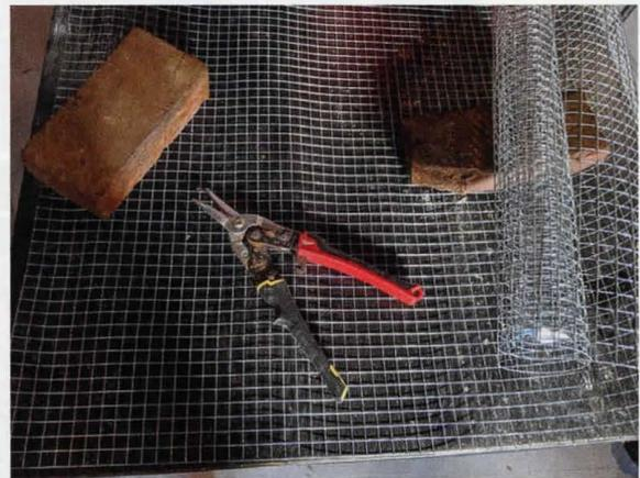
*This is all you need to make a simple and inexpensive mouse guard. The hardware cloth is readily available at hardware stores. You'll want  $\frac{1}{2}$ ". The bricks are there simply to keep the wire from rolling back on itself.*
