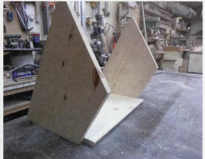
*Lay the first side on the bench and attach the end with glue and screws. Turn, and attach the other end. (This is a top bar nuc, so very short).*
