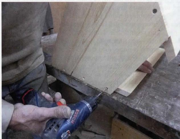
*Attach the other end. See how the sides stick down below? Use your entrance reducer or a 1½" stick to get the proper spacing.*
