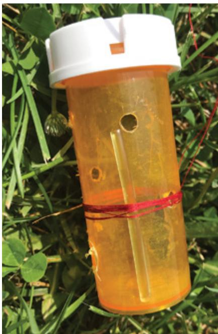
*Drone Lure: The lure is a pill bottle with holes drilled into it. There is an artificial queen pheromone stick inside the bottle. The lure hangs on a thread about 20 feet below the flying UAV.*
