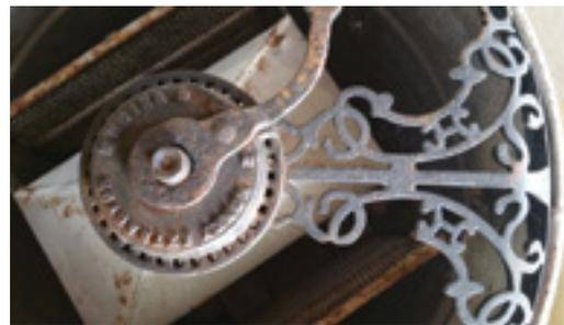
the models that were made between 1879 and 1892. However A.I. made 10 models of extractors that used that bracket. In 1893 the top crank was changed as the filigree bracket kept breaking. Thus many of these extractors became unusable because the bracket and crank were parts that could not be replaced. There were over 10,000 extractors in use. I copied some of the pages out of three of the catalogs that tell of the different models and the use of the extractors.
