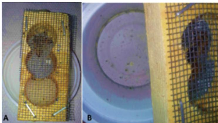
**Figure 2.** Modified cage is placed above a small water container (A), and the feces inside the water (B).
