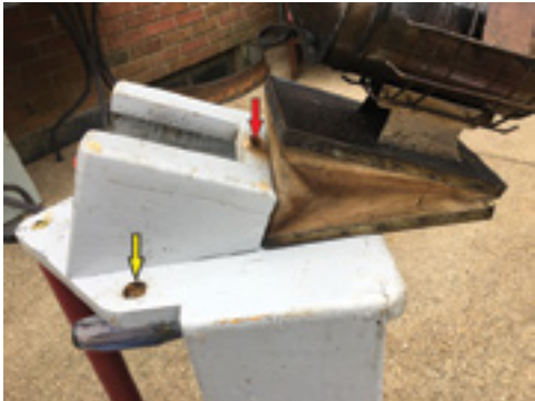
Figure 11. Smoker bracket with smoker. Note that the side gusset of the bracket is the same size as the side of the smoker bellows. Also note the hole drilled in the face of the bracket (red arrow) – this hole matches up to the air hole on the smoker and bellows and allows the smoker to be pumped while sitting in the bracket. The hole in the end of the toolbox (yellow arrow) holds the smoker cork when not in use.
