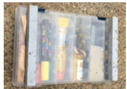
Figure 9. Wooden rails attached to the bottom of the tackle box (screwed from the inside of the box) are spaced so that they fit snugly inside of the sides of the tool box.
