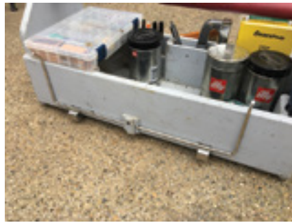
Figure 5. Slots cut through the tool box side allow the frame hanger to rest flat against the side of the box.
