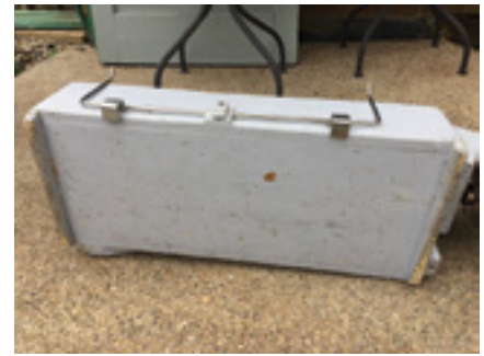
Figure 6. I attached feet at either end of the box to provide clearance for the flange of the frame hanger, which extends slightly below the bottom of the tool box.
