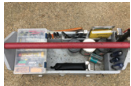
Figure 3. Slots along the inside side wall of the box are sized to hold my notebook and stapler; a block at the end of the slots is drilled to hold markers and pens.
