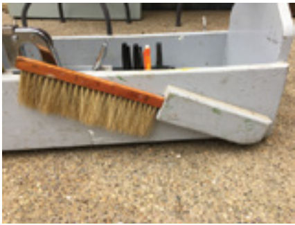
Figure 4. The holder for the bee brush is sized to fit the brush handle and angled upward to keep the brush from falling out.
