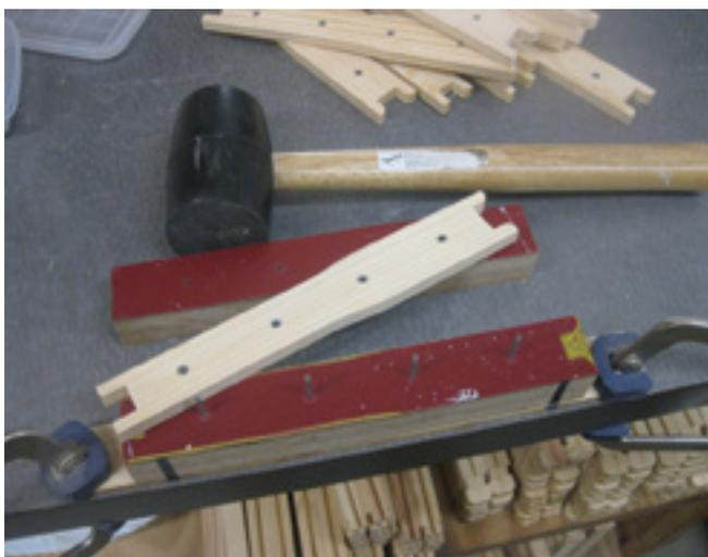
*The Eyelet Jig can be made with a saw, drill, and hammer. Use the end bar for your measurements.*
