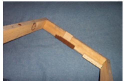
**Step 5:** Glue and nail the pieces cut in step #4 to the end pieces of the horizontal frame support.
