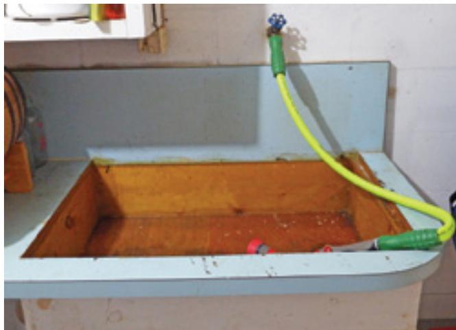
*Great for wax and tool cleaning, the wooden sink box mounts flush with counter from below and was fiber glassed in. Outdoor style spigot with garden hose and sprayer provides water.*
