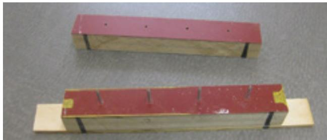
*The end bar eyelet jig. Bottom made with nails spaced to fit end bar and base to hold nails in jig and hold jig in place on workbench. Top anvil with holes to marry bottom anvil nails.*
