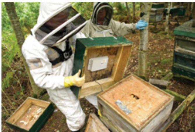
ApisProtect's sensor and battery package.
