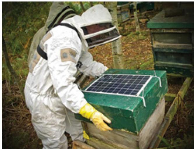
*Solar cells recharge the batteries in the ApisProtect sensor unit.*
