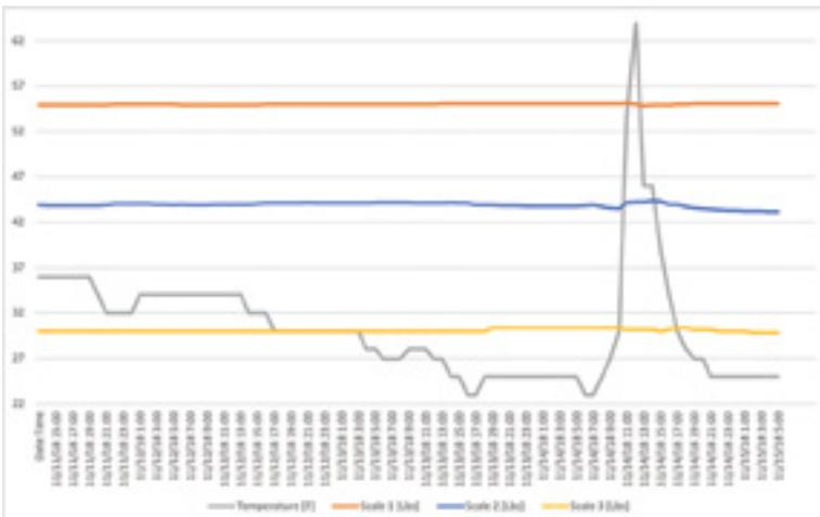
**Figure 5.** The impact of temperature on weight captured from a stack of scales. Actual weight subjected to each unit is constant, but degree to which the load cells are compensated for temperature varies.
