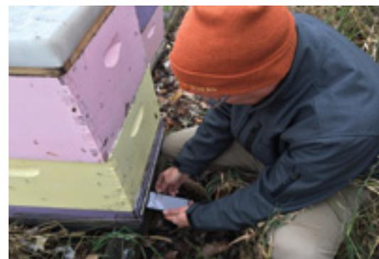
**Figure 3.** One of the authors collects data from a Solution Bee scale that uses Near field communication (NFC).
