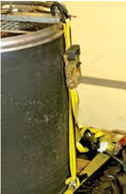
*Ratchet straps being used to secure extractor to the trailer bed.*
