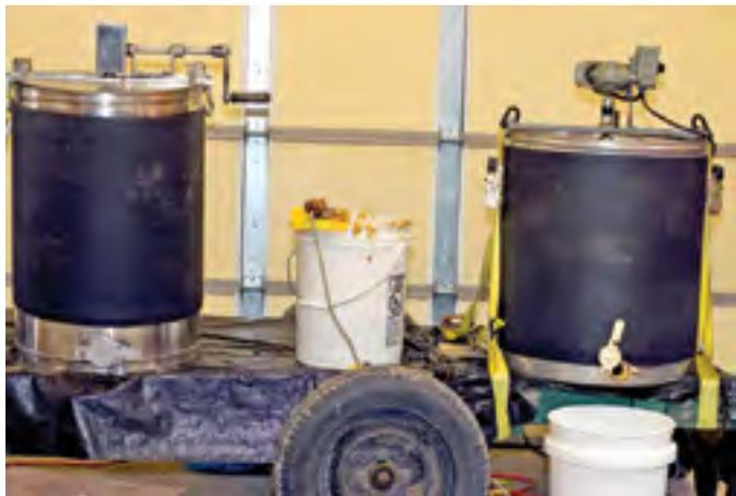
A heated holding tank and a small heated extractor.
