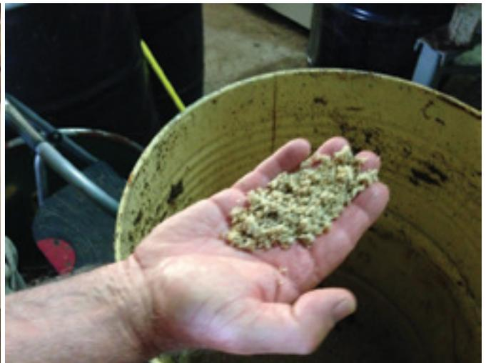
*Wax flakes out of the separator.*
