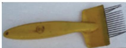
Bent and missing tines
