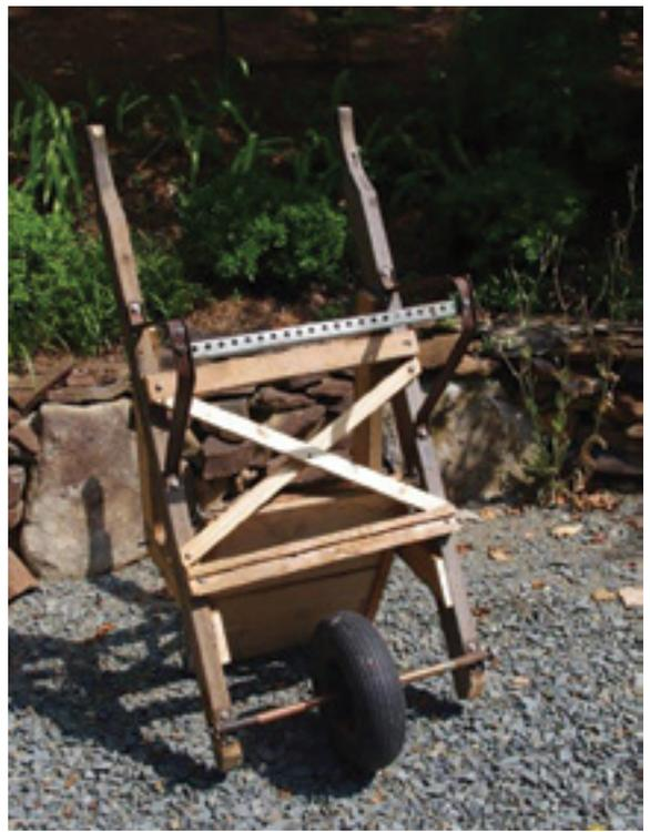
*FIRMING THINGS UP: Field testing demonstrated that an additional diagonal brace was needed to hold the frame square. Here is the underside with the final bracing applied.*
