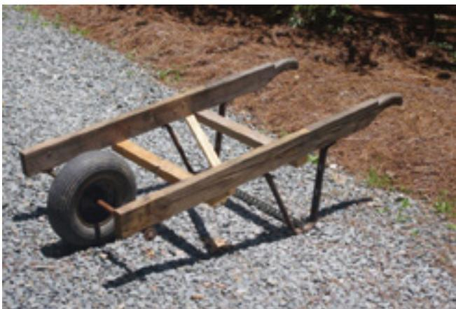
*OFF THE BENCH AND ONTO THE GROUND: With the basics done, I can get a feel on how comfortable the unit is to lift and push. Field test will show the need for another diagonal brace.*
