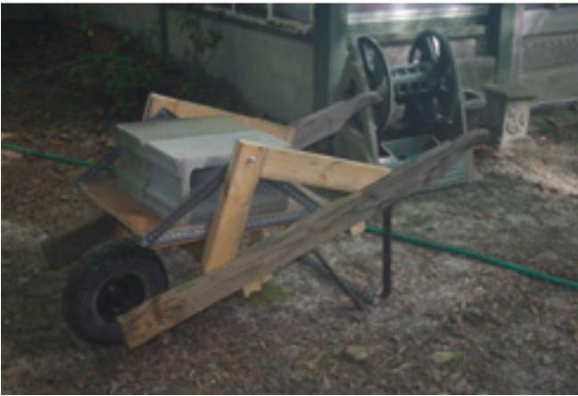
*FIELD TEST: Loading the carrier with a few cinder blocks showed that front and rear platform lips are needed as material will move with vibrations from bumps in the terrain.*
