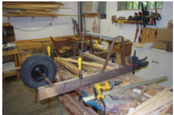
*START SQUARE, STAY SQUARE: The frame is set square to my square workbench with four clamps. Now I can pre-bore and attach other pieces confident the cradle will rock without binding on the frame.*
