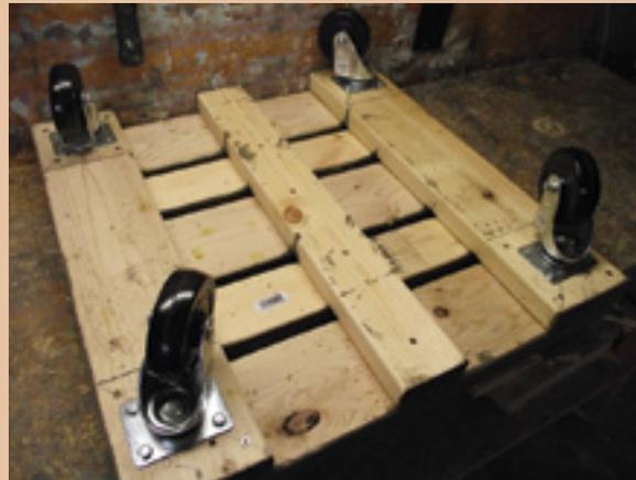
**Step 8:** Position the base so the bottom is up (3 boards). Then add the castors using the lag screws (part #3). Be sure to leave enough room between the lag screws and the ends or sides of the boards to prevent splitting when the castor wheels hit a rough spot which causes stress on the lag screws.
