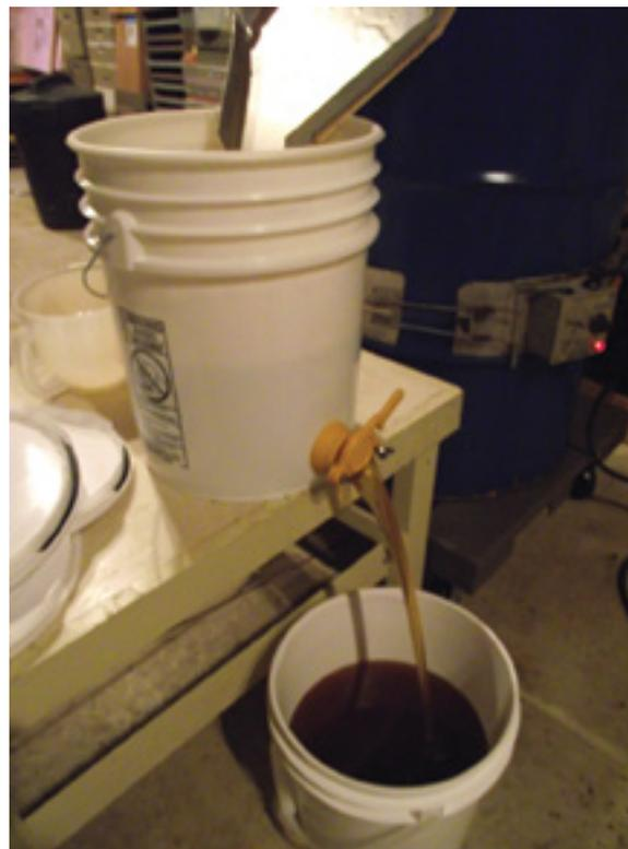
**Problem #8** – solved – To bridge this gap I built a chute made of ¾" wood covered with aluminum. The sides are turned up to keep the honey in the chute and
