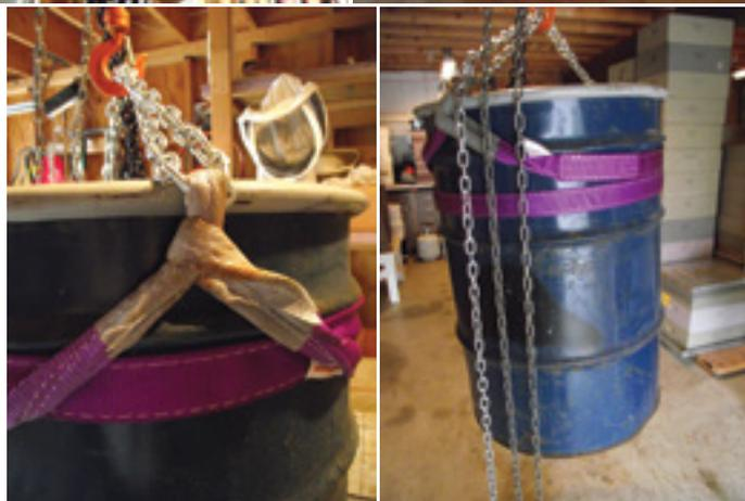
**Problem #6** – Problem #4 revisited and solved – To unload the drum we acquired a 1,000 lb. chain hoist and suspended it from the loft in the barn. Although I was sure the loft floor could handle a 700 lb. static load, I wasn't about to test my calculations. I cut a hole in the loft floor and added a five foot 1.5" pipe across the floor joists. This distributed the load across four floor joists. I was confident this would work, but I also kept my fingers crossed.
