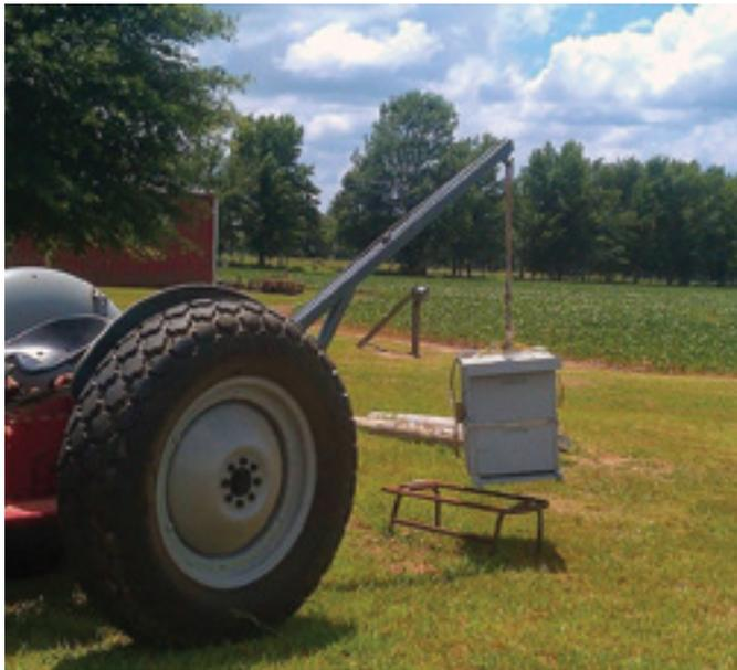
Hydraulic lift being used to pick up a hive. (photo credit – Red Belly Farm, Mississippi)
