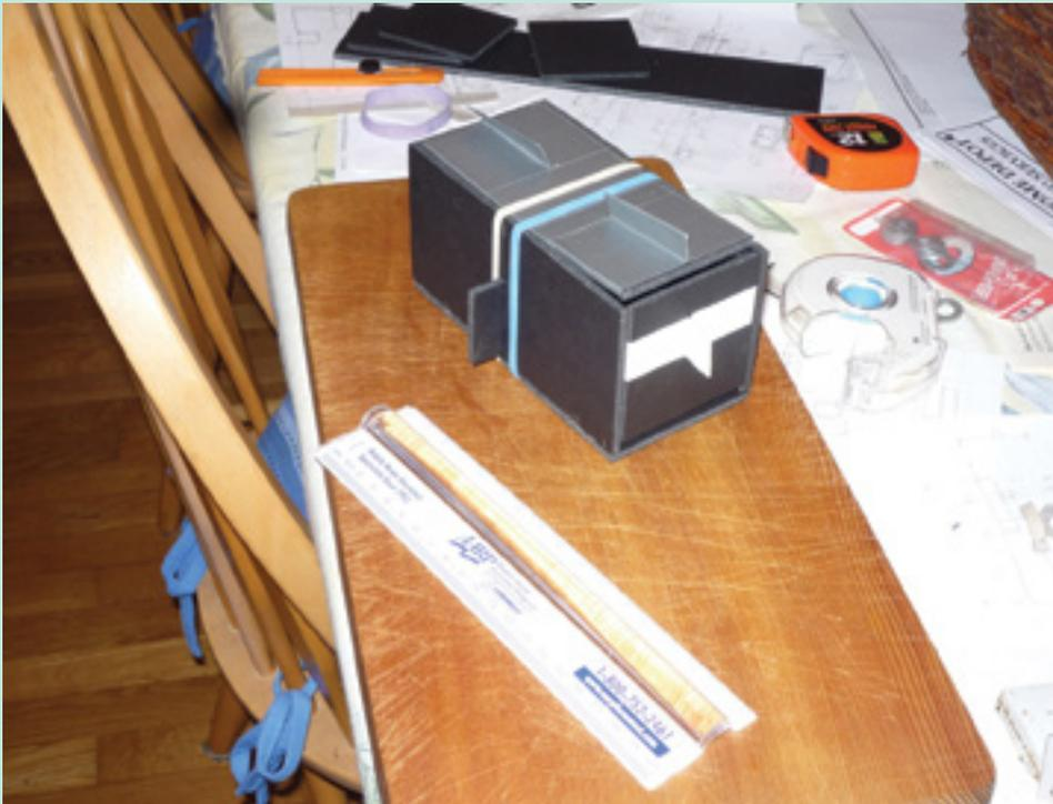
**Figure 1.** Beeline box made with foam core board, Plexiglas, and duct tape. The foam core board pieces are glued together. The Plexiglas top and its hinged covers are fastened with rubber bands. Hinges are duct tape.
