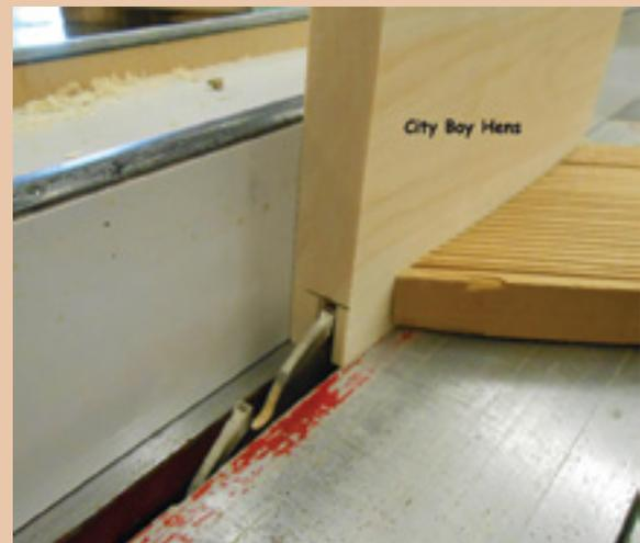
Next, lower the blade to 3/8" and adjust the rip fence so that there is 3/4" distance from the *left* side of the blade to the fence.
