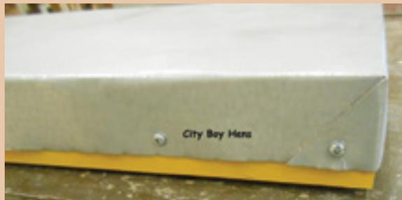
Now, screw those edges to the sides of the cover with #6 x 1/2" pan head metal screws.
