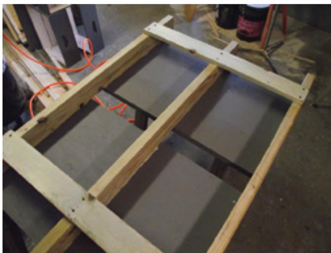
**Step 5:** Turn the pallet over and using construction adhesive and screws add the standoff stiffeners (parts #7) to the bottom of the pallet. In addition to stabilizing the standoffs they provide the support when a pallet is stacked on top of another set of hives. These stiffeners are set 5" back from the front of the standoffs and provide extra stability to the pallet.
