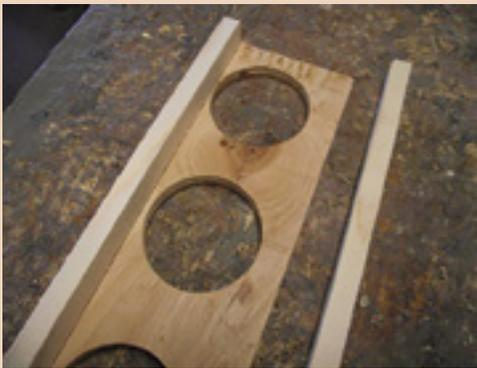
**Step 7:** Glue & nail or staple (parts #2) to the bottom of the base. It is easiest to nail from the top through the plywood into the leg. Use one nail or staple on each corner of the hole to ensure a solidly attached leg.
