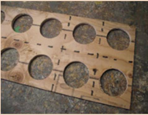
**Step 5:** Once the holes are drilled, cut the plywood in half lengthwise.
