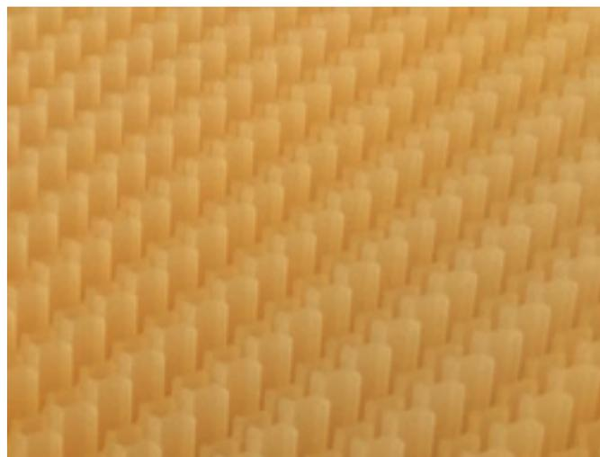
The two rows that make up a cell are not flush at the face of the frame.
