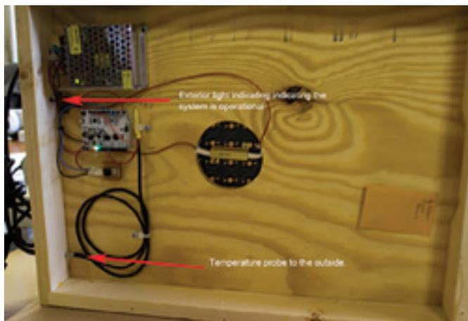
Heat generating device and temperature probes.
