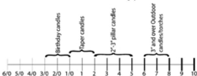
**Square Braid Wick Sizes** – Wick graphic: Although this is not completely correct in terms of actual diameter of wicking, it gives an overall picture of relative sizes, commonly available wick sizes and the range of uses.
